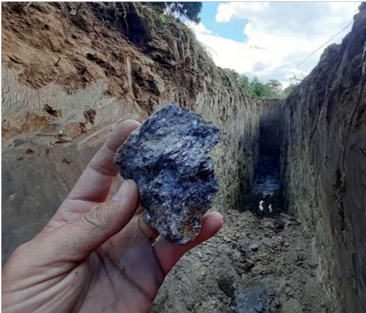
Figure 7.3 Graphite mineralisation exposed by Gratomic Inc. trench CGT001 (20 to 22 m) grading 21.65 % TGC from the southern part of the Capim Grosso Project (source: QP).
