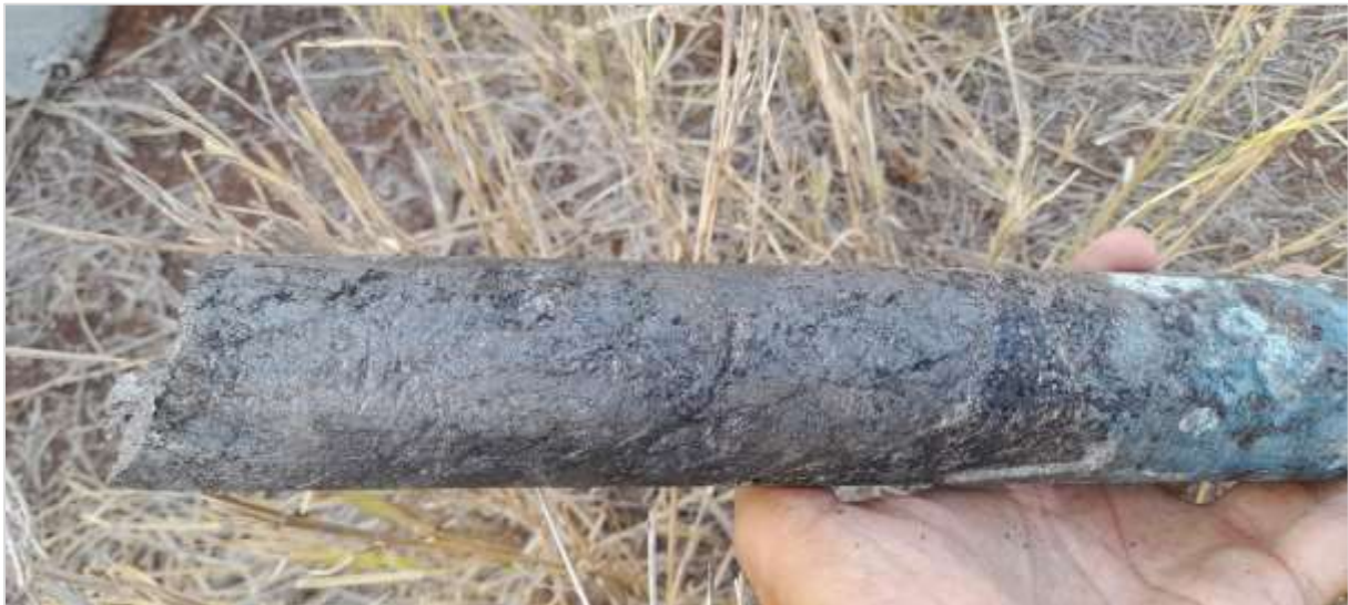
Figure 7.7 Graphite mineralisation from the Gratomic drilling on the Capim Grosso Project (source: QP).
