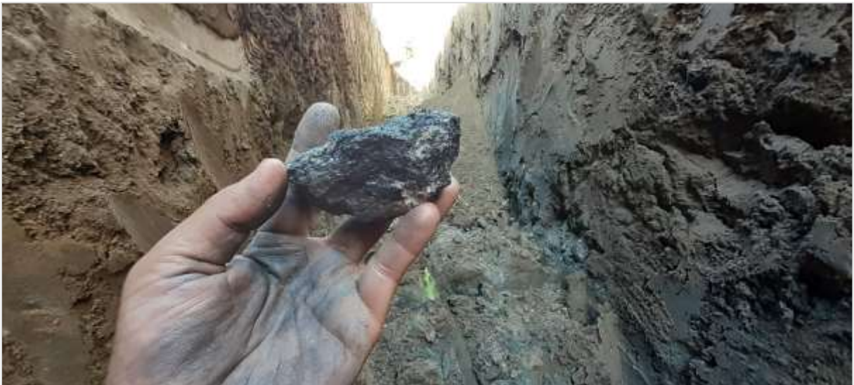
Figure 9.3 Most of the trenches excavated were able to penetrate up to 2 or 3 m in depth and most intersected graphite mineralization (Source: QP).
