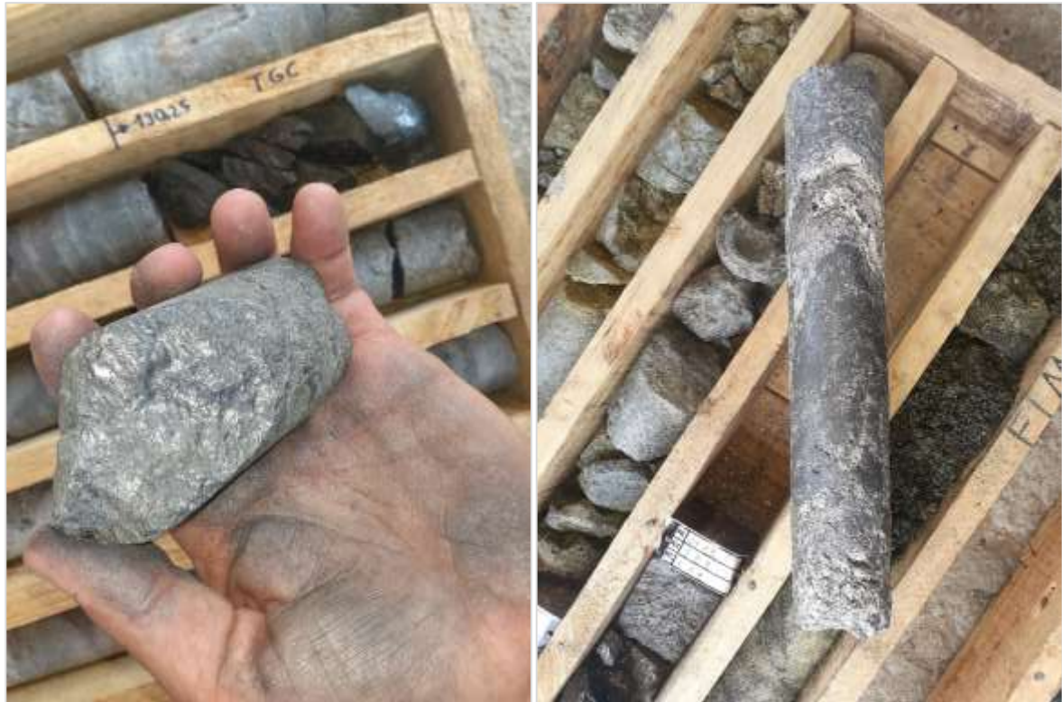
Figure 7.6 Graphite mineralisation from the Gratomic drilling on the Capim Grosso Project (Drillhole CGD002 130.25 m tot 130.69 m containing mineralisation of 8.42 % TGC) (source: QP).
